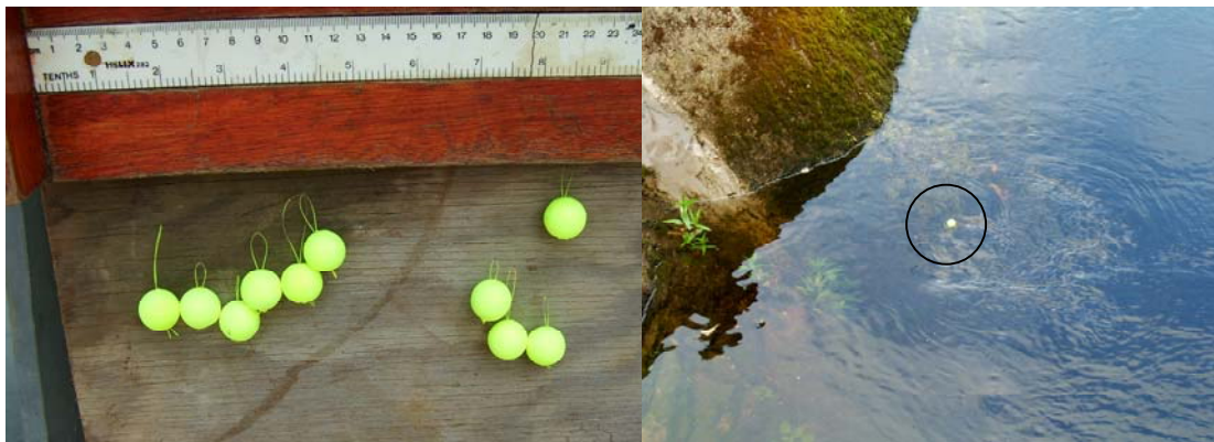
Plate 7.5 Fluorescent polystyrene float tags as used to follow close-range movements in front of screens and bywashes. The left-hand photograph shows a number of floats prior to attachment; the right hand side shows one as viewed in the water (inside black circle).
