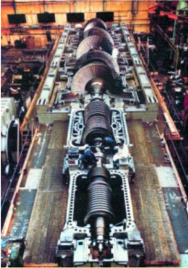
Figure 2-1 Internal view of a 500 MWe turbine. Small-diameter HP cylinder is in the foreground, then an intermediate pressure cylinder and three LP stages. Overall length of unit is 55 metres and large LP disc (blades) diameter is 2.5 metres.
